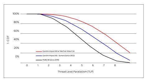
Figure 2.2. CPU TLP demand for mobile game trend and concurrent case based on Dimensity 9300
