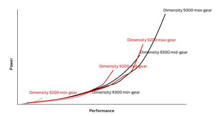
Figure 4.2. Multi-gear CPU power efficiency and performance curve comparison between Dimensity 9300 and 9200
