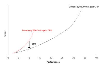
Figure 4.1. Min-gear CPU power efficiency curve comparison between Dimensity 9300 and 9200
