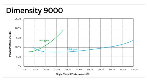
Figure 3.2. Dimensity 9000 CPU power efficiency
