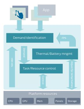
Figure 5.1. Closed-loop scheduling in the system
