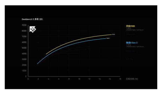
Figure 4.3. Geekbenchv5 multi-core: Dimensity 9300 achieves better power efficiency than Qualcomm Snapdragon 8 Gen 3
