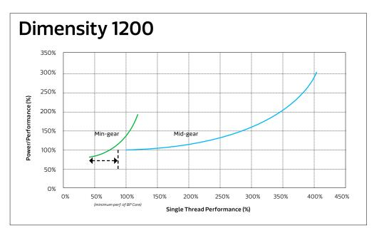
Figure 3.1. Dimensity 1200 CPU power efficiency
