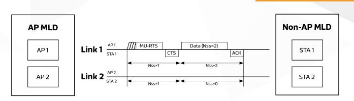
Figure 6. Downlink Transmission from STR AP to EMLSR STA (Max. NSS=2)
