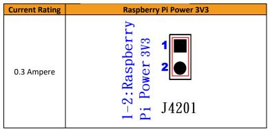
Figure 3-5. Jumper Selection for Raspberry Pi Power 3V3 Input
