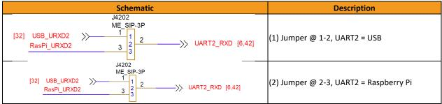
Figure 3-7. Configure UART2 Ports
