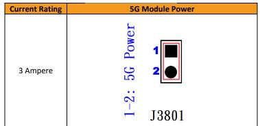
Figure 3-4. Jumper Selection for 5G Module Power Input
