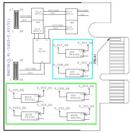
Figure 4-5. Block Diagram of D6 Camera Board
