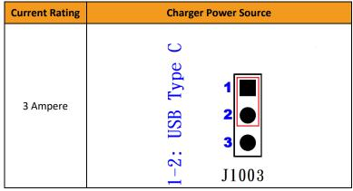
Figure 3-2 Jumper Selection for Charger Power Source Input Path
