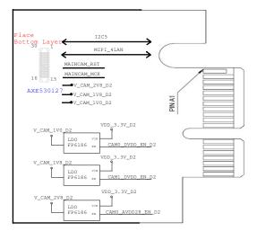
Figure 4-3. Block Diagram of D2 Camera Board
