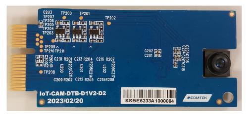
Figure 4-2. D2 Camera Board
