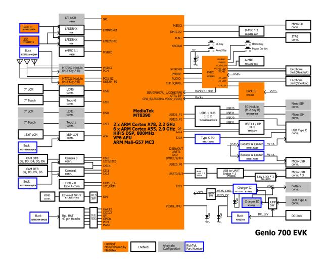
Figure 1-1. Genio 700 Evaluation Kit System Block Diagram
