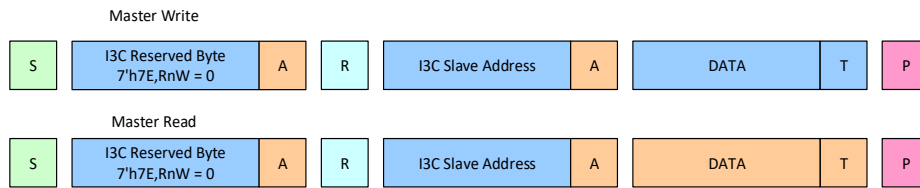
Figure 3-103 I3C SDR Private Write/Read
