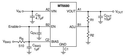
Figure 4-1. Soft-start delay using an RC circuit to enable the device
