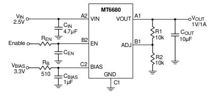
Figure 1-3. Typical application circuit
