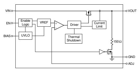
Figure 5-1. MT6680 functional block diagram
