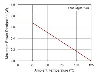
Figure 4-2. Derating curve of maximum power dissipation
