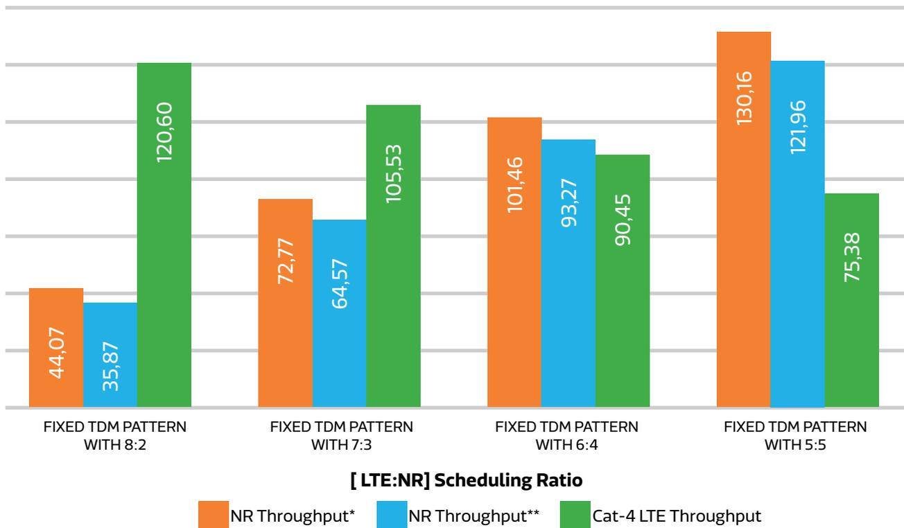
Figure 21. NR and LTE Downlink Throughput (Mbps) in DSS Operation with Different TDM Patterns
