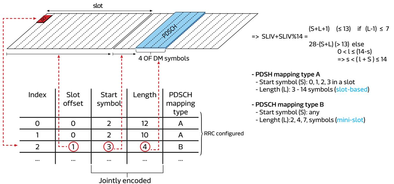
Figure 5. NR PDSCH Mapping Types in Time Domain
