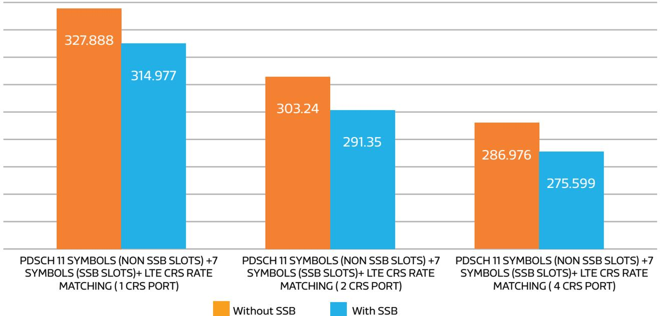
Figure 13. Maximum NR Slot Throughput (Mbps) for Case #3
