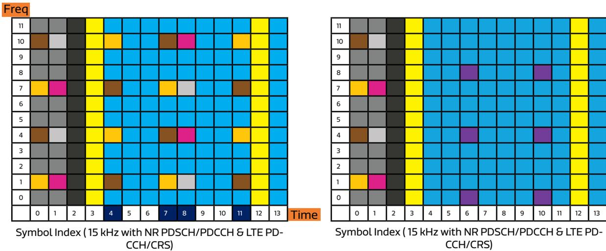
Figure 22. NR PDSCH Scheduling with LTE CRS Rate Matching in non-MBSFN subframes
