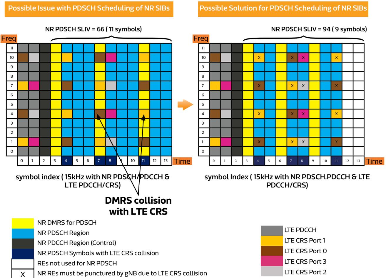
**Figure 10. Impact of DSS on NR PDSCH and DMRS Resource Mapping in SA Deployment**
