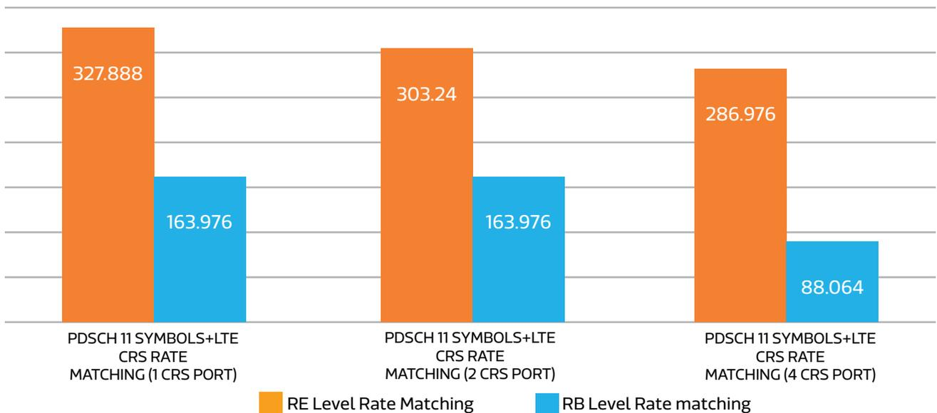
Figure 12. Maximum NR Slot Throughput (Mbps) for Case #2 – RE vs RB Level CRS Rate Matching
