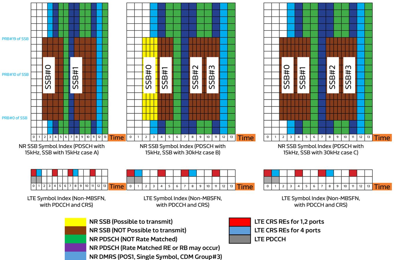
Figure 2. Impact of Spectrum Sharing on NR SSB Channel: Non-MBSFN
