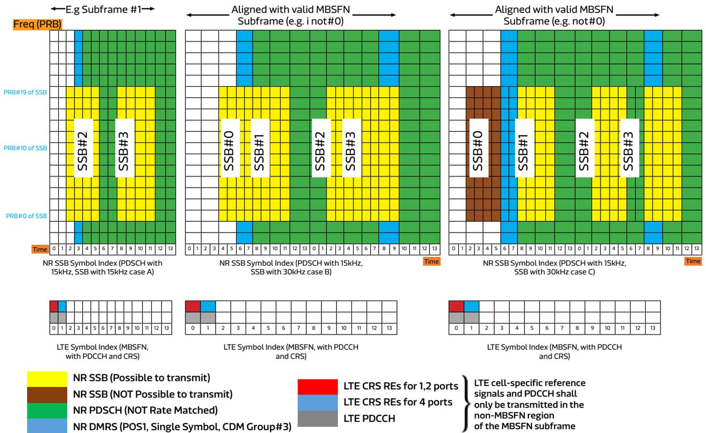
Figure 3. Impact of Spectrum Sharing on NR SSB Channel: MBSFN
