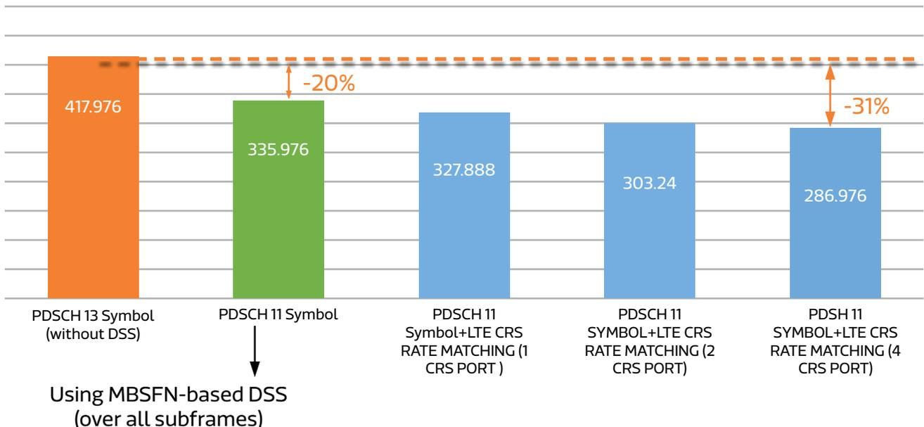
Figure 11. Maximum NR Slot Throughput (Mbps) for Case #1
