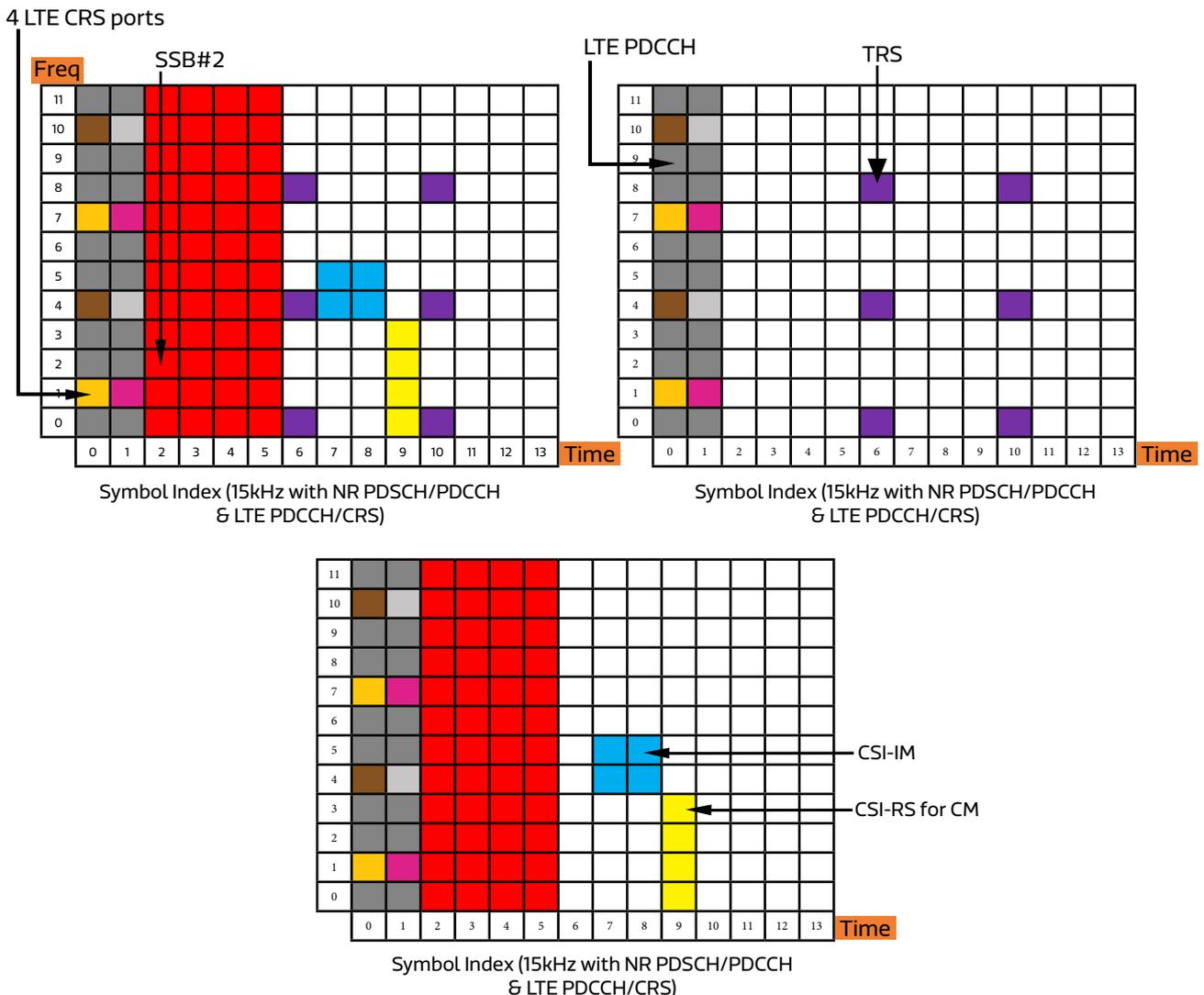
Figure 20. Overall View of NR and LTE Reference Signals in Time-Frequency
