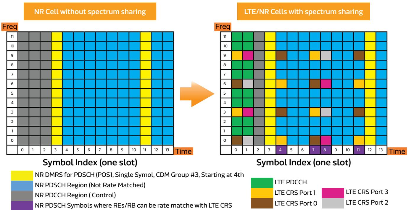
Figure 6. NR PDCCH/PDSCH SCS=15 kHz (without SSB)
