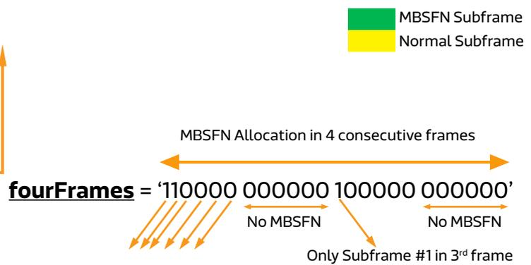
Subframes #1, #2, #3, #6, #7, and #8 are allocated to MBSFN if their bitmap is set to "1" in the *fourFrame* over the period of four frame, and then the pattern repeats where it was left, based on the frame number in the table for frames satisfying:
