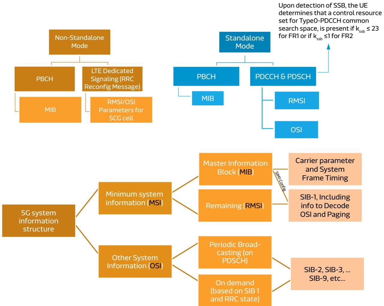
Figure 9. System Information in 5G NSA vs. SA Deployment
